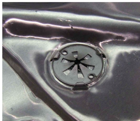
Picture 2 : Heatshield Fastener –Clipping instead of screwing
