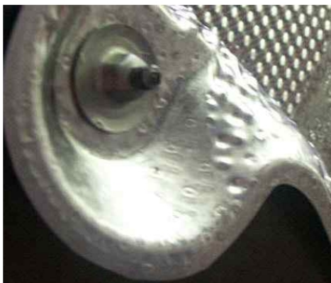
Picture 2 : Heatshield Fastener –Clipping instead of screwing
